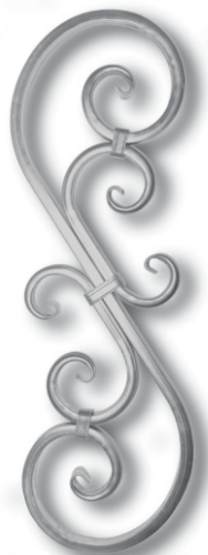
Model: M214 10 1/4" W X 29 1/2" H Mtl. 5/8" sq. tube 18 gauge
